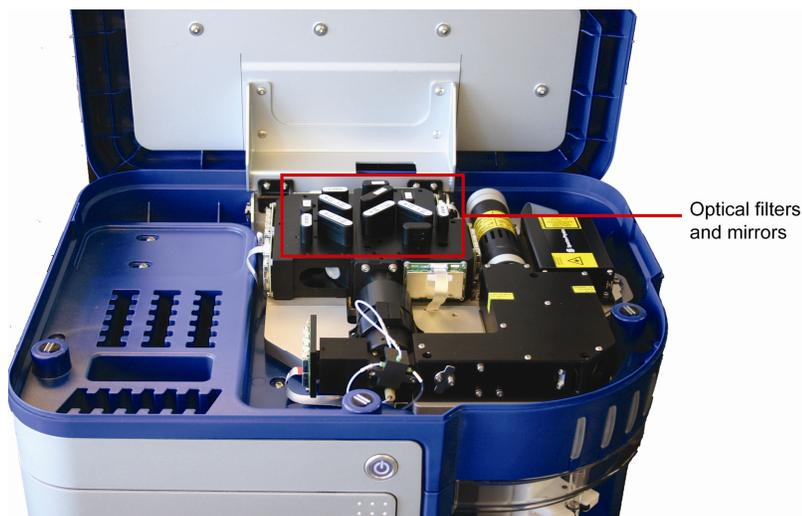
2. Remove the optical holder containing the appropriate filter or mirror.
