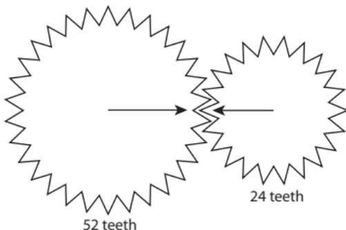
How many revolutions must the large gear make before the arrows line up again?
