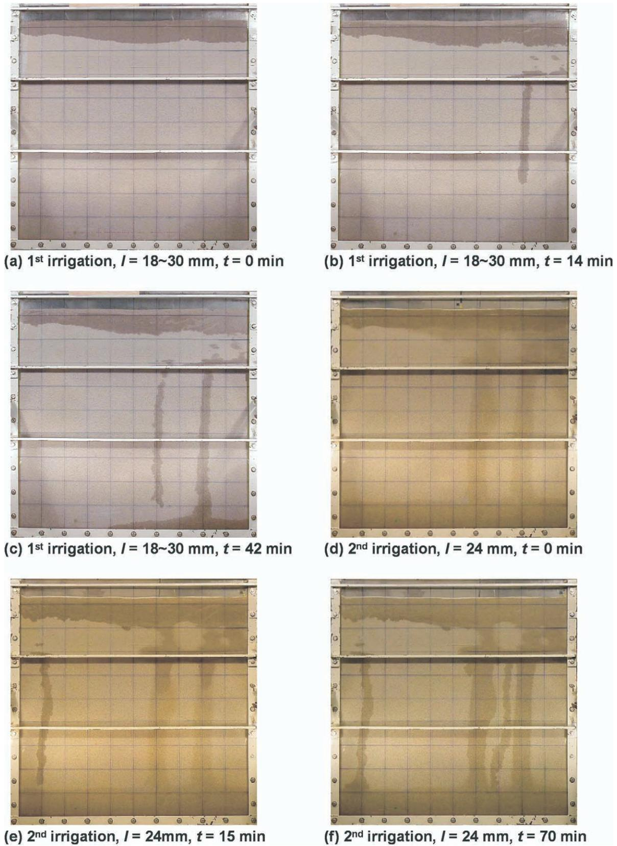
Fig. 6. Redistribution of unevenly applied water in a finer sand (top 22 cm) and a coarser sand (below) through a line source.  $I$  is the depth of water applied into the sands, and  $t$  is the time of redistribution.
