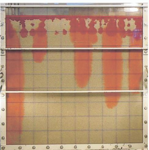
(e) 5<sup>th</sup> irrigation,  $l = 24\text{mm}$ ,  $t = 2\text{ min}$
