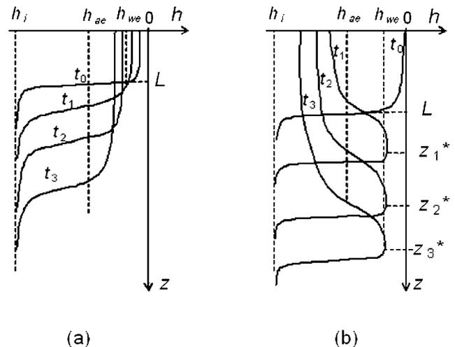
**Fig. 3.** Schematic matric potential profiles,  $h = h(z, t)$ , at the end of infiltration ( $t = 0$ ) and at different times  $t$  during redistribution: (a)  $L < S$  and (b)  $L > S$ . The asterisked variables indicate the positions of the maximum water content at the time (Peck, 1971).
