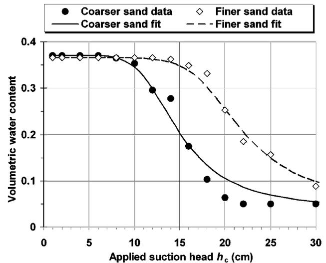
Fig. 5. Drying retention curves of the experimental materials.
