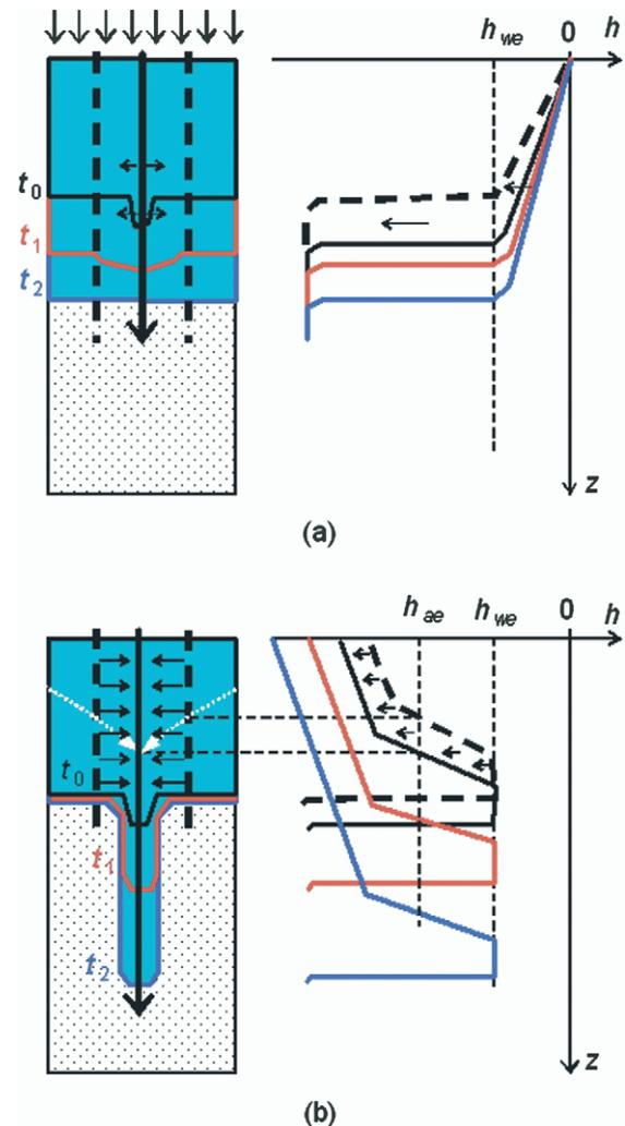
Fig. 4. Evolution of a perturbation at the wetting front during (a) ponded infiltration and (b) redistribution. The arrows show the flow directions.
