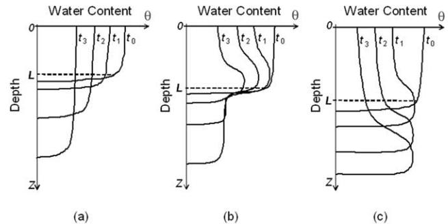
Fig. 1. Types of possible redistribution profiles after ponded infiltration.
