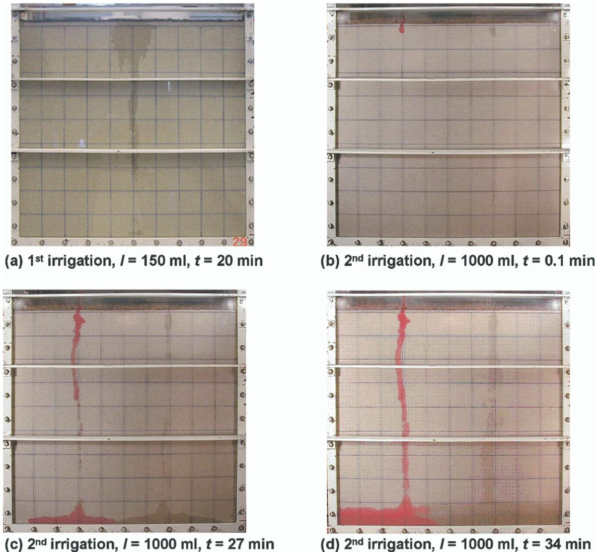
Fig. 7. Redistribution of fluids in the coarse sand: (a) deaired water ( $\rho = 0.993$ ) added instantaneously; (b) through (d) salty water with anionic red dye ( $\rho = 1.06$ ) and deaired water through an irrigation dropper ( $1 \text{ drop s}^{-1}$  or  $6.6 \text{ mL min}^{-1}$ ).  $I$  is the depth of water applied into the sands, and  $t$  is the time of redistribution.
