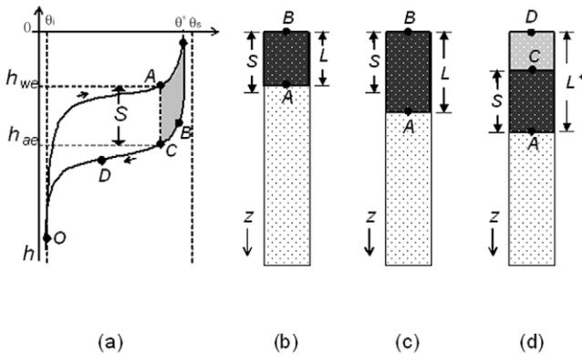
**Fig. 2.** Schematics of moisture and pressure redistribution with respect to the amount of initial application: (a) hysteresis effects, (b)  $L < S$ , (c)  $L > S$ , and (d) water blob at the front. The asterisked variable indicates the maximum water content of the profile during redistribution (Peck, 1971).
